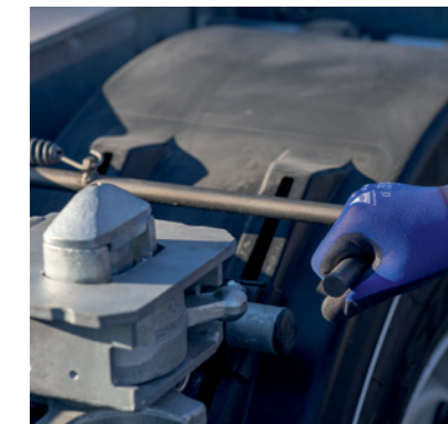
Manual locking for pneumatic rear extension.
