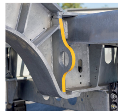
The container trailer chassis is equipped with ferry lashings as standard for use with ferry transport.
