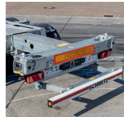
The rear extension extends pneumatically to the selected container position. For 45' containers - pull-out underride guard.
