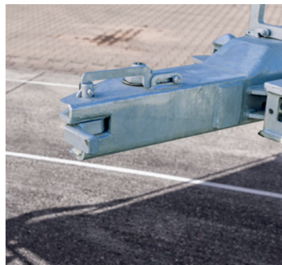
Patented MULTI LOCK on the front beam in locking position for tunnel container with sloping corners.
