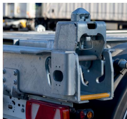
Two STEP LOCKS® on the rear extension allow you to adjust your semitrailer/container chassis in a matter of moments.
