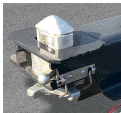
Standard TWIST LOCK locking mechanism: retractable and with anti-rotation lock
