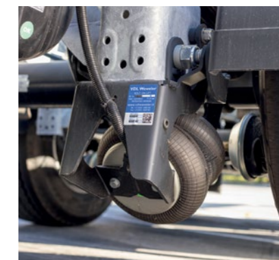
The lift axle* as a starting aid extends the wheelbase and thus increases the pressure on the drive axle. Unloaded and in the lifted position, tyre wear is reduced.
