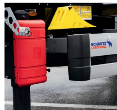
New side collision protection and fire extinguisher* on the support structure.
